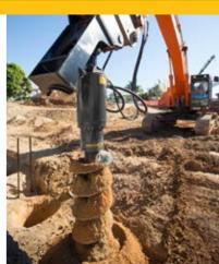
**SUITABLE FOR 8 - 22 TON EXCAVATORS**
