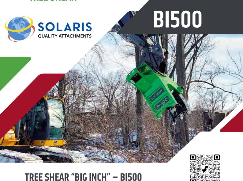
BI500 is the real game changer for big projects. Developed for excavators from 23 t to 40 t, with 110 t cylinder of force, BI500 is able to provide a 24" cutting diameter.
