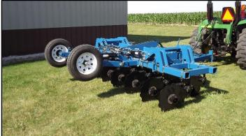
The Solaris SCX Straw Crimper's discs can pivot left and right and up and down independently, leaving a well-secured, even mulch installation
