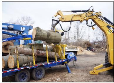
The Solaris-Black Splitter S2, S2X, SG1 & SB hydraulic wood splitter attachments are designed to fit all models of excavators up to 12 ton, backhoes and skid-steers. The unique rotating threaded cone provides extremely efficient wood-splitting power for various timber types including hard, soft, straight, knotty and twisted.
